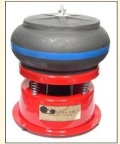
For polishing jewelry the vibratory tumbler is not recommended over the rotary tumbler for tumbling the jewelry with steel shot. The vibratory tumbler is good for sanding and smoothing jewelry castings such as rings. Plastic or ceramic media is usually used for this purpose.
