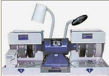
**Step 1:** Remove the splash hoods and water pans. Clean the Nova wheel surfaces with soapy water. Thoroughly rinse and dry. Finish cleaning the surfaces with an acetone-soaked cloth.
