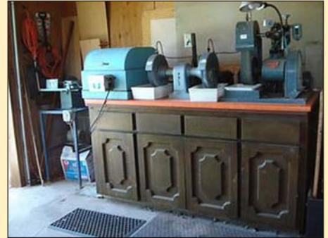
The trim saw in the left corner is on its own stand, and is from Crown Lapidary Equipment; its floor space is 18" by 20".
